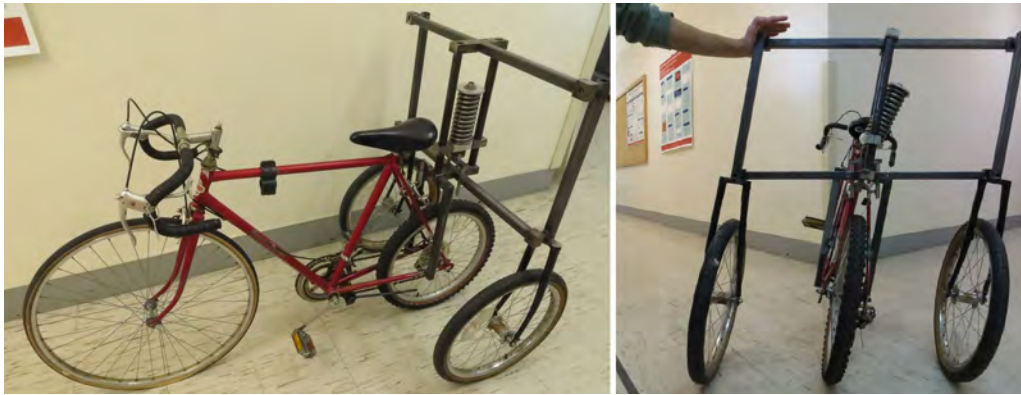
Figure 1. A ‘bricycle’: a vehicle which can transition between bicycle and a tricycle. It is a bicycle with two extra ‘training’ wheels at the back on a spring-loaded parallelogram mechanism. The spring resists bicycle lean, more or less depending on its adjustment. When the spring is removed the training wheels are mechanically invisible, effectively reducing the bricycle to a bicycle. When the spring is locked the bicycle is effectively a tricycle. The neutral point in-between, when the spring is such that the bicycle is in equilibrium at all small angles of lean , is the main topic of study here.
